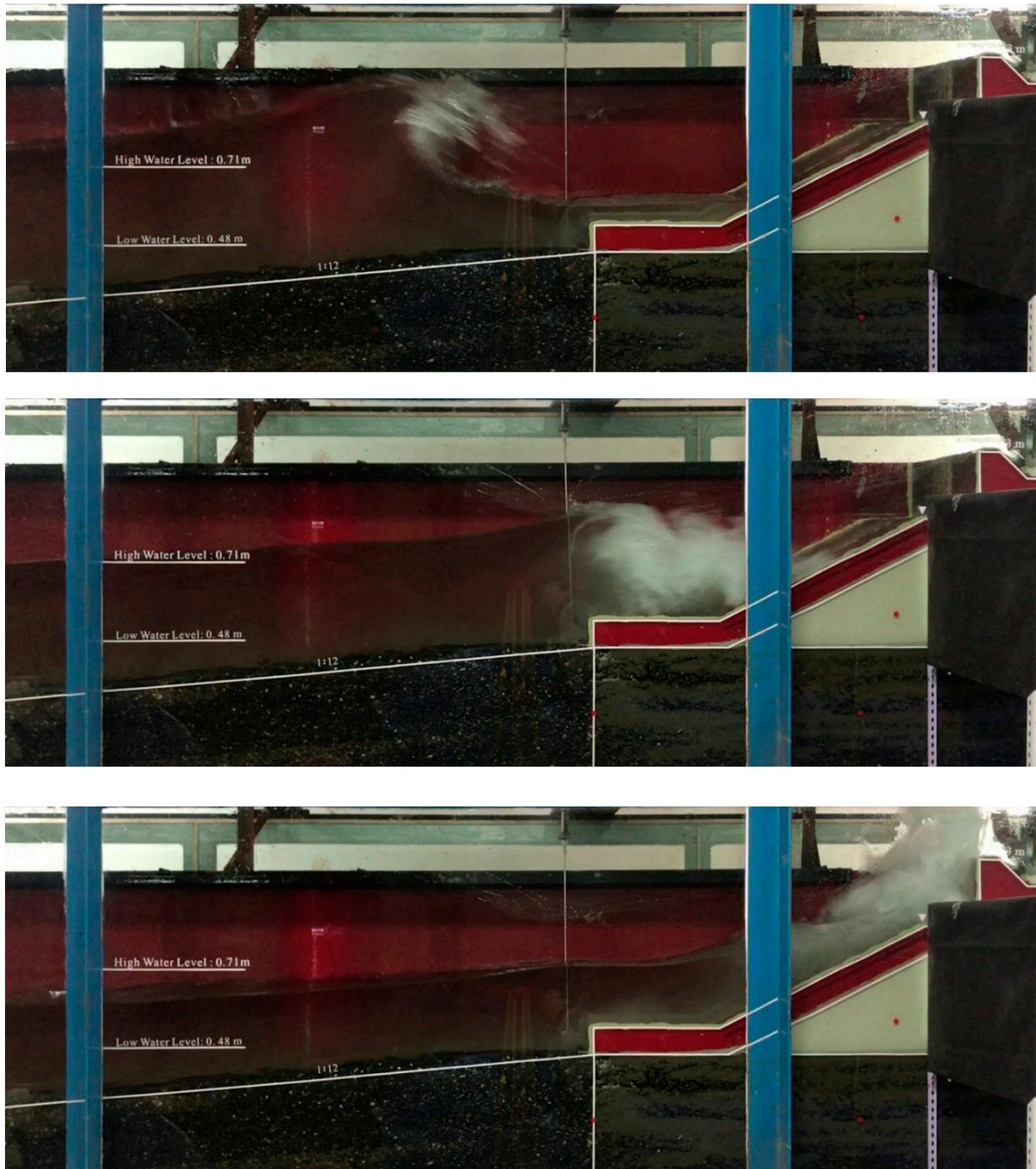
**Figure 7.** Revetment breakwater is being impacted by regular wave and water overtopping is occurring, observed in Test 3.
