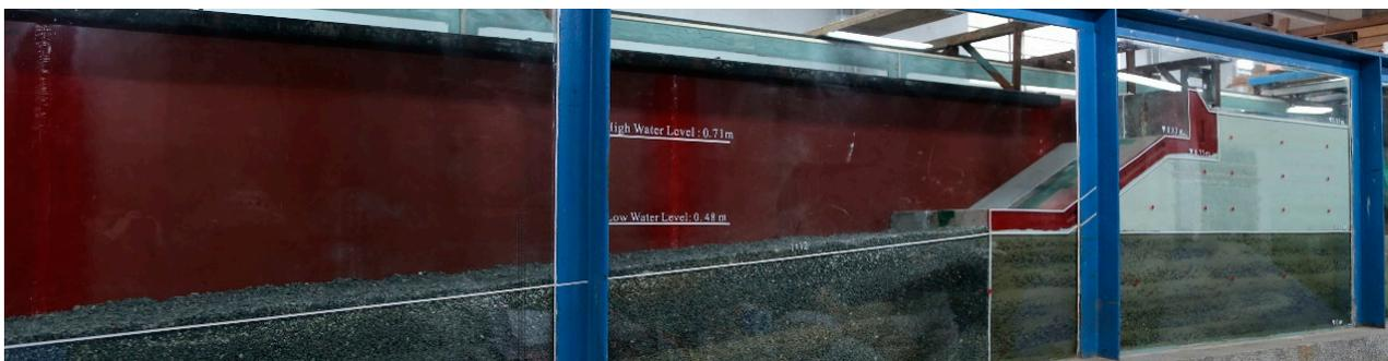
**Figure 3.** A real view of the completed physical model without accropodes or rubble in front of the revetment breakwater.
